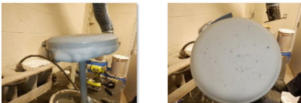
Figure 13-38 Filter Cake 59 wt% Solids Feed, 90 second Cycle Time
