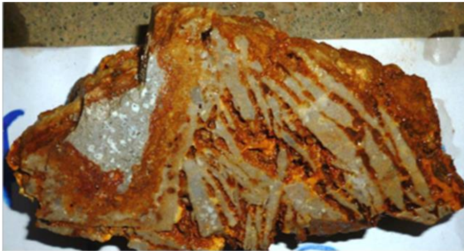
Figure 7-4. Fractured Brecciated Lithocap
